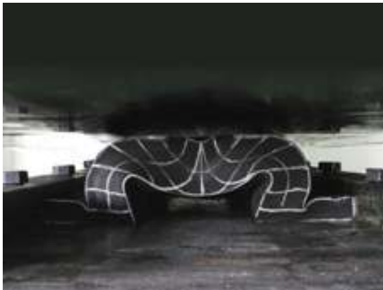
7. COMPRESSION TEST AT 45%
