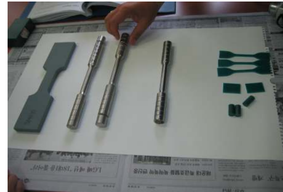
4. STEEL & UHMW-PE TEST
